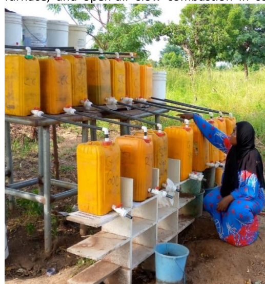
Figure 2: Anaerobic multi-chamber downwards filtration set-up. (Source: Field study, 2021; Nimatu et al., 2023) and Schematic layout of the multi-chamber downward anaerobic filtration system used to treat WW at the Zagayuri irrigation field.
