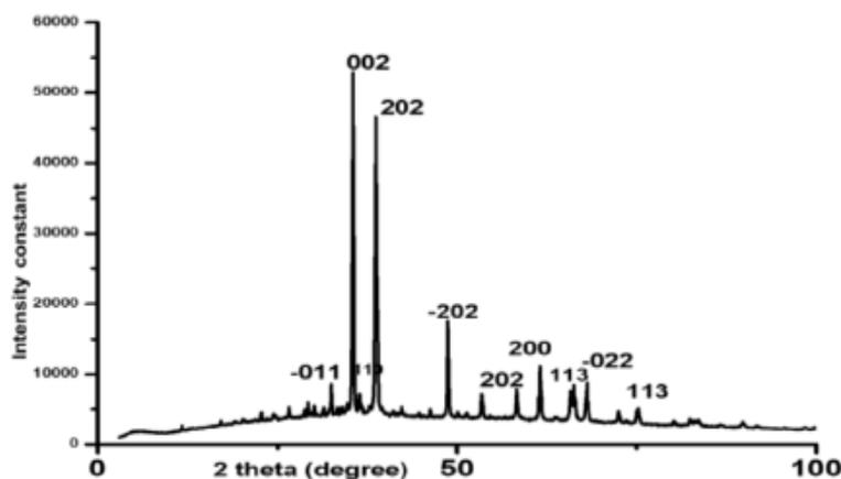
**Figure 7:** XRD spectrum of the copper oxide nanoparticle.
