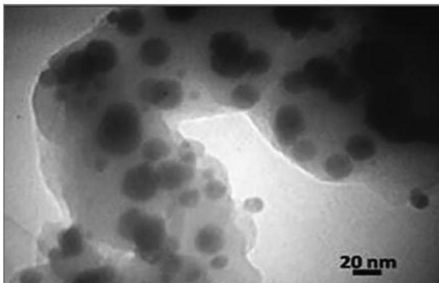
**Figure 6:** TEM image of copper oxide nanoparticles at magnification of 20µm.
