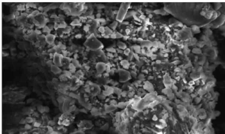
**Figure 4:** SEM image of copper oxide nanoparticles at magnification of 10 μm.
