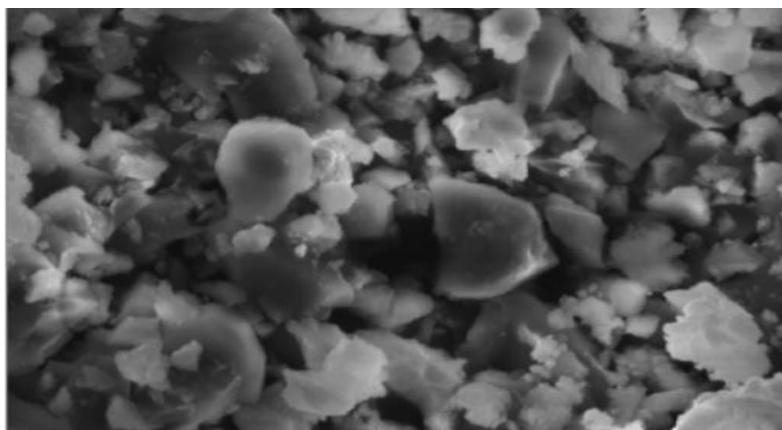
**Figure 5:** SEM image of copper oxide nanoparticle at magnification of 5μm.
