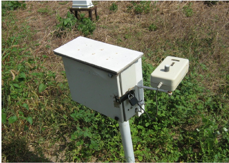
Figure 1: Picture of the Constructed Reliable Model Pyranometer
